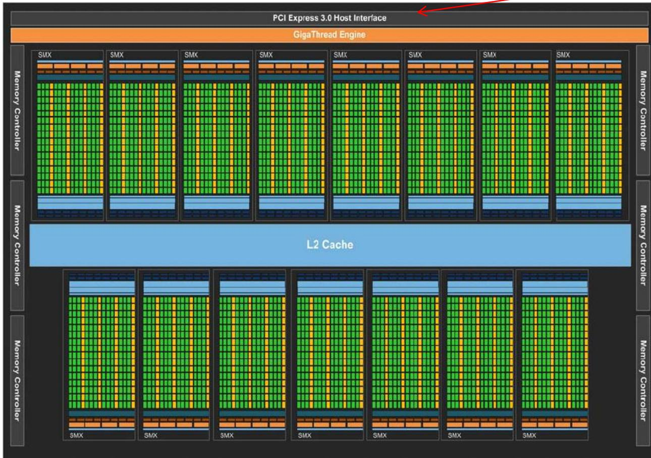
GigaThread Engine is the center of the chip, it generates and distributes blocks of threads between different multiprocessors.
